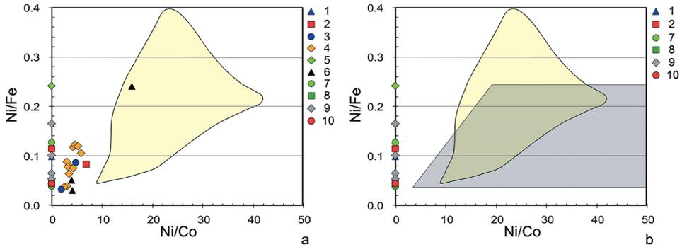
Fig. 3. Ni/Fe vs Ni/Co in welding seams; data were taken from *table 1*. The yellowish area was delimited by A. Jambon by plotting Ni/Fe and Ni/Co ratios of fresh iron meteorites (for details see *Jambon 2017a*): a – compositions of virtually all welds are displaced to lower Ni/Co ratios; b – the grey area corresponds to possible plotting if the undetermined cobalt content would be within the range of 0 to 1 %.
