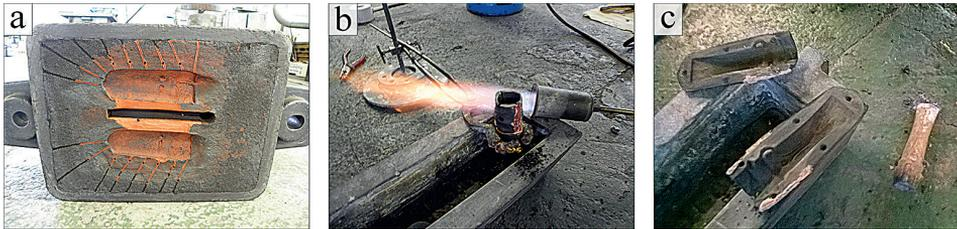
Fig. 11. The stages of the experimental casting of the Przedmieście type axe compatible with the casting mould from Elgiszewo: a – casting the mould; b – pre-heating the mould; c – knocking the casting out of the mould.
